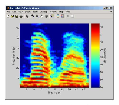
In this example, you viewed the spectrogram of your speech signal using a Matrix Viewer block. You can find additional Signal Processing Blockset examples in the Help browser. To access these examples, click the Contents tab, double-click Signal Processing Blockset, and then click Examples. A list of the examples in the Signal Processing Blockset documentation appears in the right pane of the Help browser.
