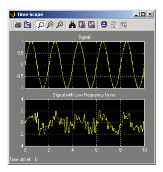
You have now built a digital filter and used it to model the presence of colored noise in your signal. This is analogous to same as modeling the low frequency noise reaching the microphone in the cockpit of the aircraft. Now that you have added noise to your system, you can experiment with methods to eliminate it. In the next section, "Adaptive Filters" on page 4-9, you design an adaptive filter to remove this noise from your signal.
