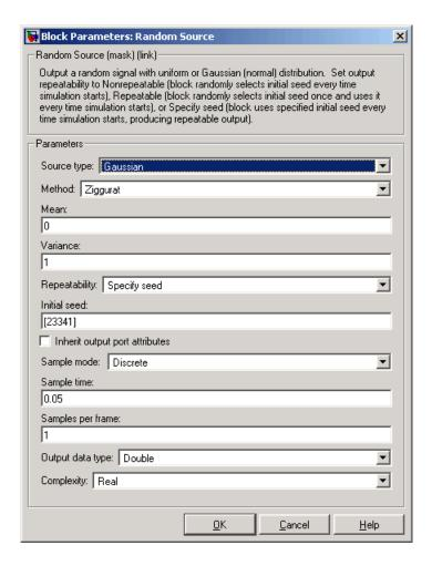
Opening this dialog box causes a running simulation to pause. See "Changing Source Block Parameters During Simulation" in the online Simulink documentation for details.
