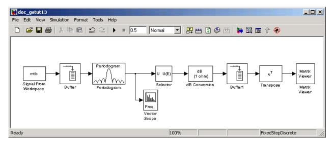
**2** Run the model. During the simulation, the **Vector Scope** window displays a sequence of power spectrums, one for each window of the original speech signal. The power spectrum is the contribution of every frequency to the power of the speech signal.
