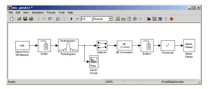
Once you have assembled the blocks needed to view the spectrogram of your speech signal, you can set the block parameters. To learn how to do this, see "Setting the Model Parameters" on page 6-13.
