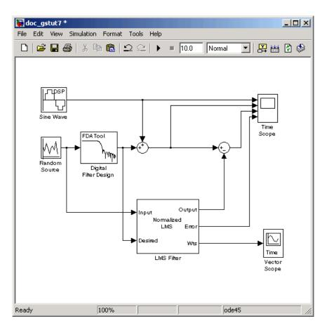
6 Set the configuration parameters. Open the Configuration Parameters dialog box by selecting Configuration Parameters from the Simulation menu. In the **Solver** pane, for the **Stop time** parameter, enter inf. From the **Type** list, choose Fixed-step. From the **Solver** list, choose discrete (no continuous states).
