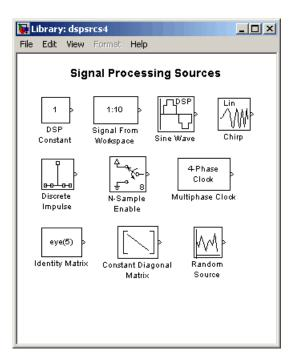
4 Click-and-drag a Sine Wave block into your new model. The Sine Wave block generates a sinusoidal signal.
