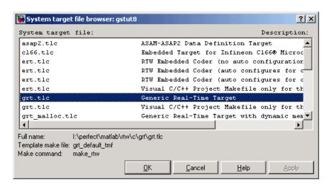
The **Real-Time Workshop** pane now displays the correct system target file (grt.tlc), template makefile (grt\_default\_tmf), and make command (make\_rtw).
