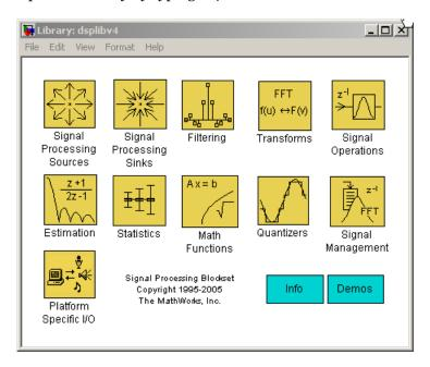
**2** Double-click the Signal Processing Sources library. The library displays the blocks it contains. You can use the blocks in the Signal Processing Sources library to create discrete-time or continuous-time signals.
