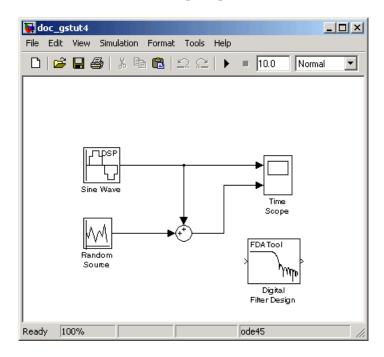
**2** Incorporate the Digital Filter Design block into your block diagram. Click-and-drag the Digital Filter Design block, and place it between the Random Source block and the Sum block.
